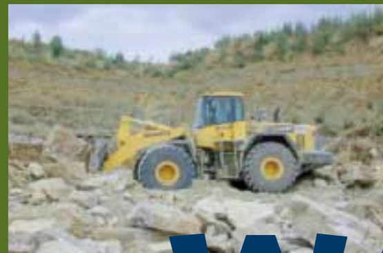
The new Komatsu WA480-5 carrying a shell-limestone block with its stone-fork for loading
