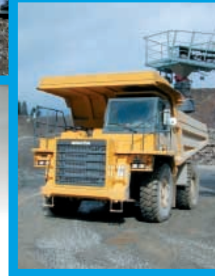
The HD325-6 transports chippings in its 24-tonne body
