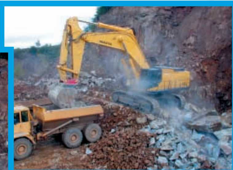
1,000 m 3 a day: the 105-tonne PC1100 SP-6 with its 4.7 m 3 bucket.
