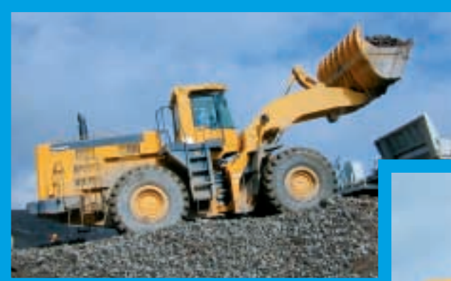
Quarry power: The WA600-3 loads blasted greywacke into a crusher.
