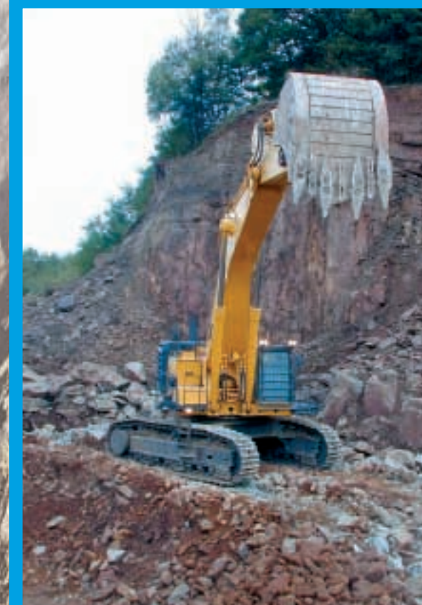
The special bucket: Hardox 700 HB wear edges and Komatsu K VX teeth size M68 and M48.
