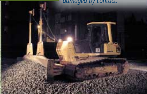
The D41 bulldozer is custom outfitted with laser sensors and a pair of front displays to tell the operator when the path is perfectly levelled.
