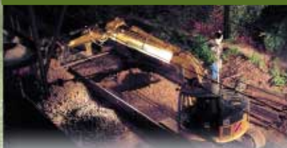
The PC128 tucks in and works comfortably under overhead wires that could easily be damaged by contact.
